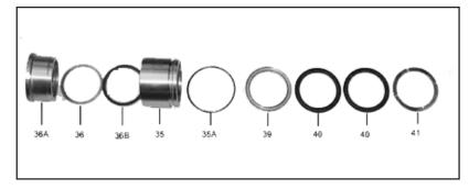
4. Remove the seal sleeve (35) from the manifold and/or crankcase. Remove the pressure rings (39&36A), v-sleeves (40&36), support ring (41) and o-rings (35A) from the manifold and seal sleeve, respectively. Examine seals carefully and replace if worn. Clean all parts.
